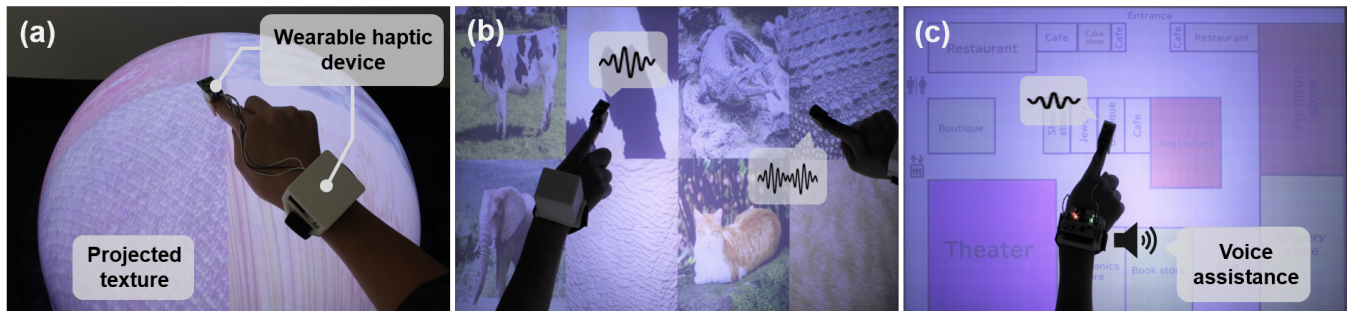
Figure 1: Application scenarios of HaptoMapping: (a) Texture design support system, (b) Visual and haptic dictionary of animals, (c) Interactive map enhanced with haptic (and audio) information for both sighted and visually impaired people.
